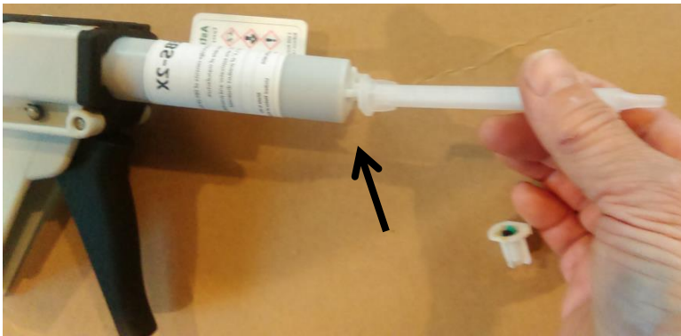
8) Slide the static mixer into the same holding slop on the cartridge
