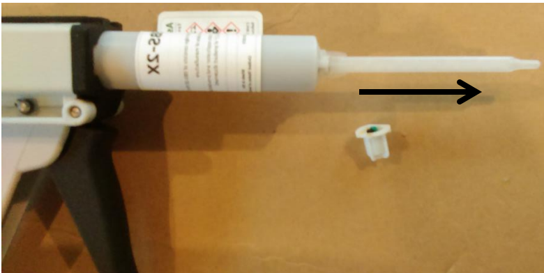
9) Start pumping the gun until the black graphite adhesive comes through the static mixer. The adhesive comes out of the mixer fully mixed
