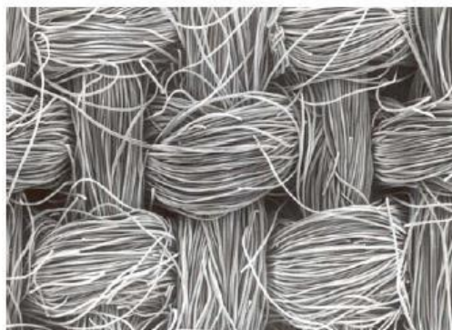
Zorflex 100% Activated Carbon Cloth in Woven Form. Magnification x40
